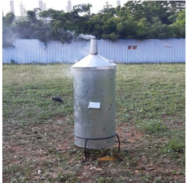
Figure 60: Pyrolysis Oven of the University of Ghana Source: Adjei-Ayim, 2022
